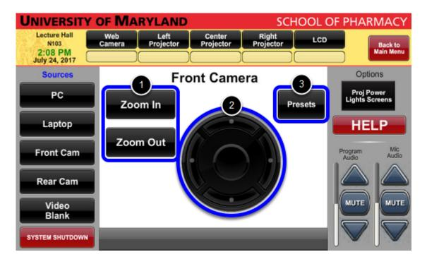
You can zoom in and out (1), pan or tilt the camera left and right or up and down with the directional wheel (2), or choose one of the preset camera locations under the "Presets" menu (3).
