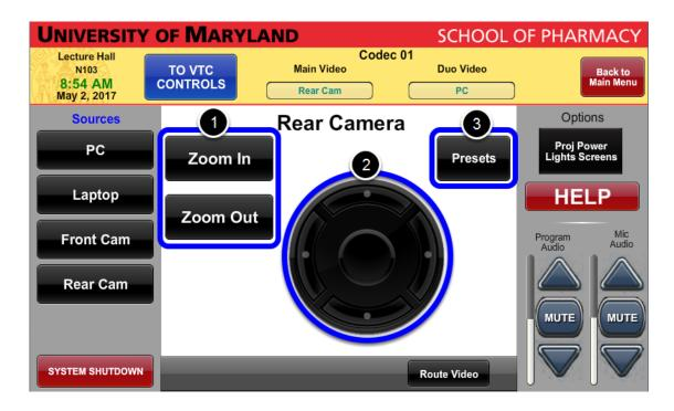
The rear camera screen gives you several options for camera movement. You can zoom in and out (1), pan or tilt the camera left and right or up and down with the directional wheel (2), or choose one of the preset camera locations under the "Presets" menu (3).
